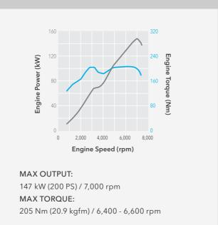
The SUBARU BOXER engine powers the SUBARU BRZ to new heights of precision and excitement. We've placed this 2.0-litre engine lower, made it more compact and moved it closer to the driver. It's the first engine of its kind to feature direct and port fuel injection technology, which enhances both its responsiveness and fuel efficiency. It's a one-of-akind design that offers a new kind of satisfaction.
